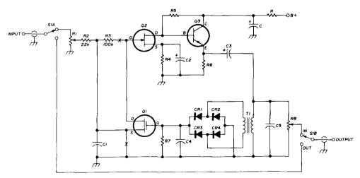
fig. 1. Basic circuit of the RP Electronics RPC-3 speech processor. Expand function is added by breaking connections between R3 and Q2 gate and between Q1 source and ground and connecting Q1 source to the junction of R2 and C1.
